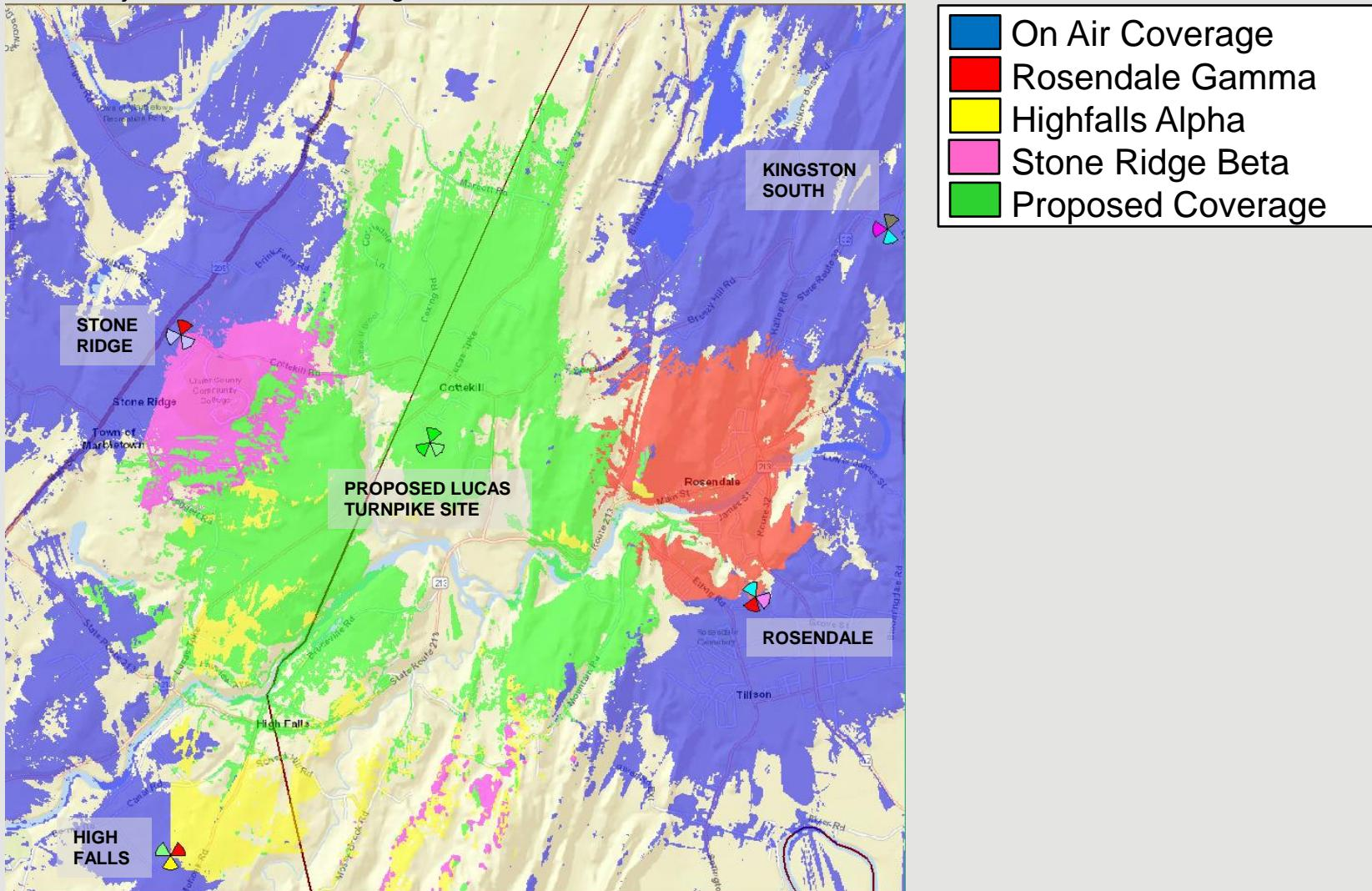
The map above adds the footprint of the proposed **Lucas Turnpike** site in green. The green best server footprint provides improved coverage and capacity throughout the identified significant gap area. This will help to resolve the coverage and capacity issues impacting the existing sectors identified in the image above.
