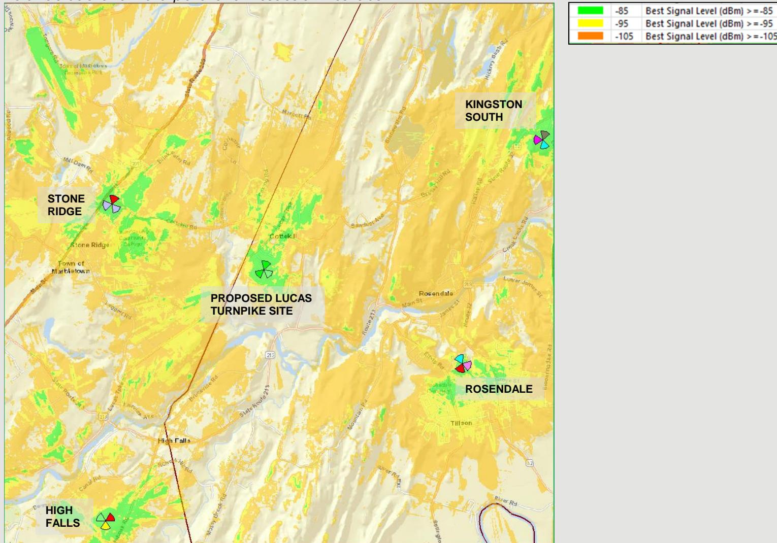
The map above adds mid band of the **Lucas Turnpike** site to the existing signal strength. The significantly improved signal strength corresponds to improved coverage and capacity throughout the identified significant gap areas. This will help to resolve the coverage and capacity issues impacting portions of the Town of Rosendale.
