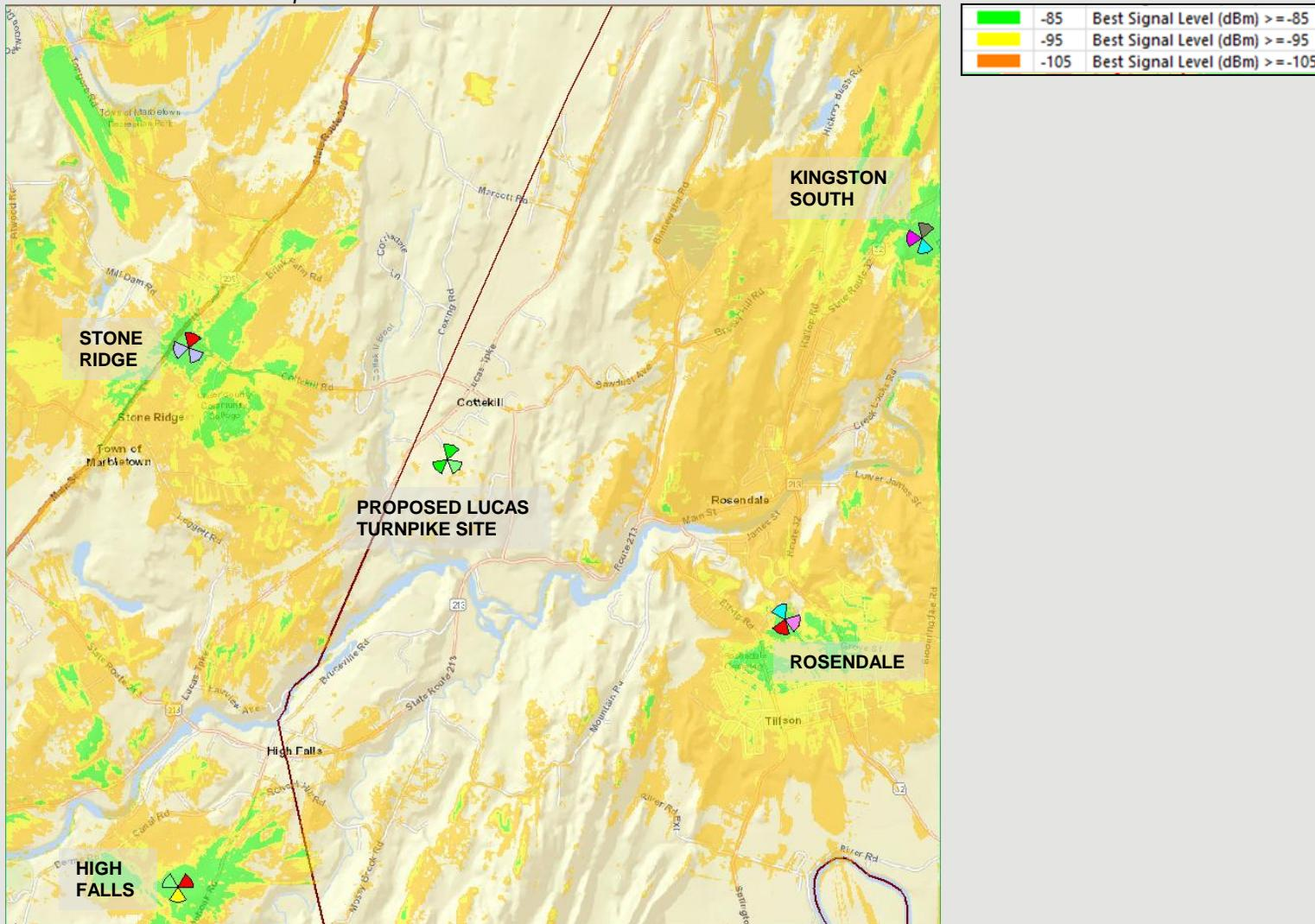
The map above represents mid band coverage from existing sites. This 2100MHz signal is very weak throughout the project area. Additional mid band network densification is required to resolve these conditions.
