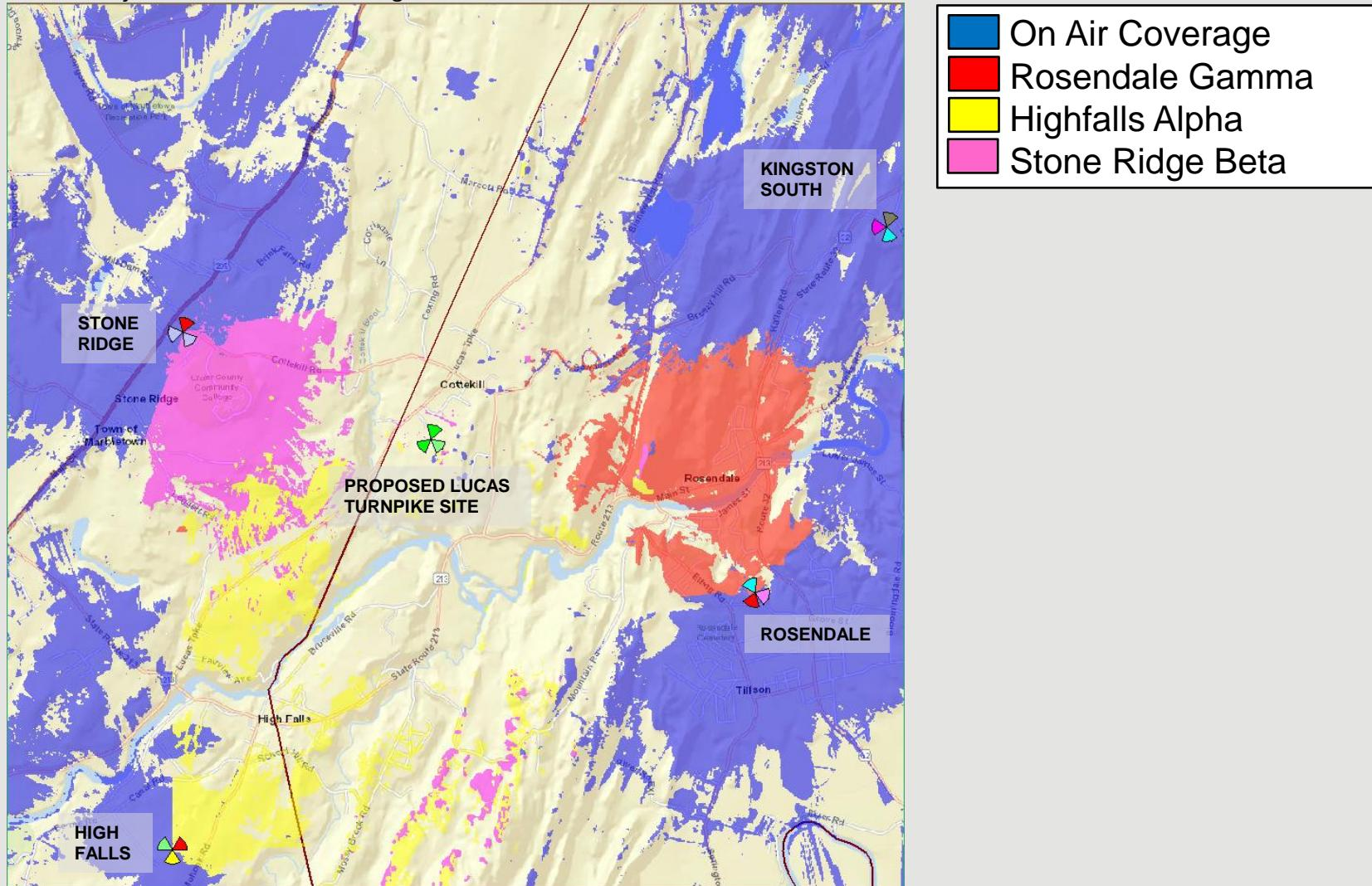
The map above represents coverage from existing sites, with the sites in need of capacity offload detailed in the legend above. Blue coverage is from other on air (Mid Band) sites.
