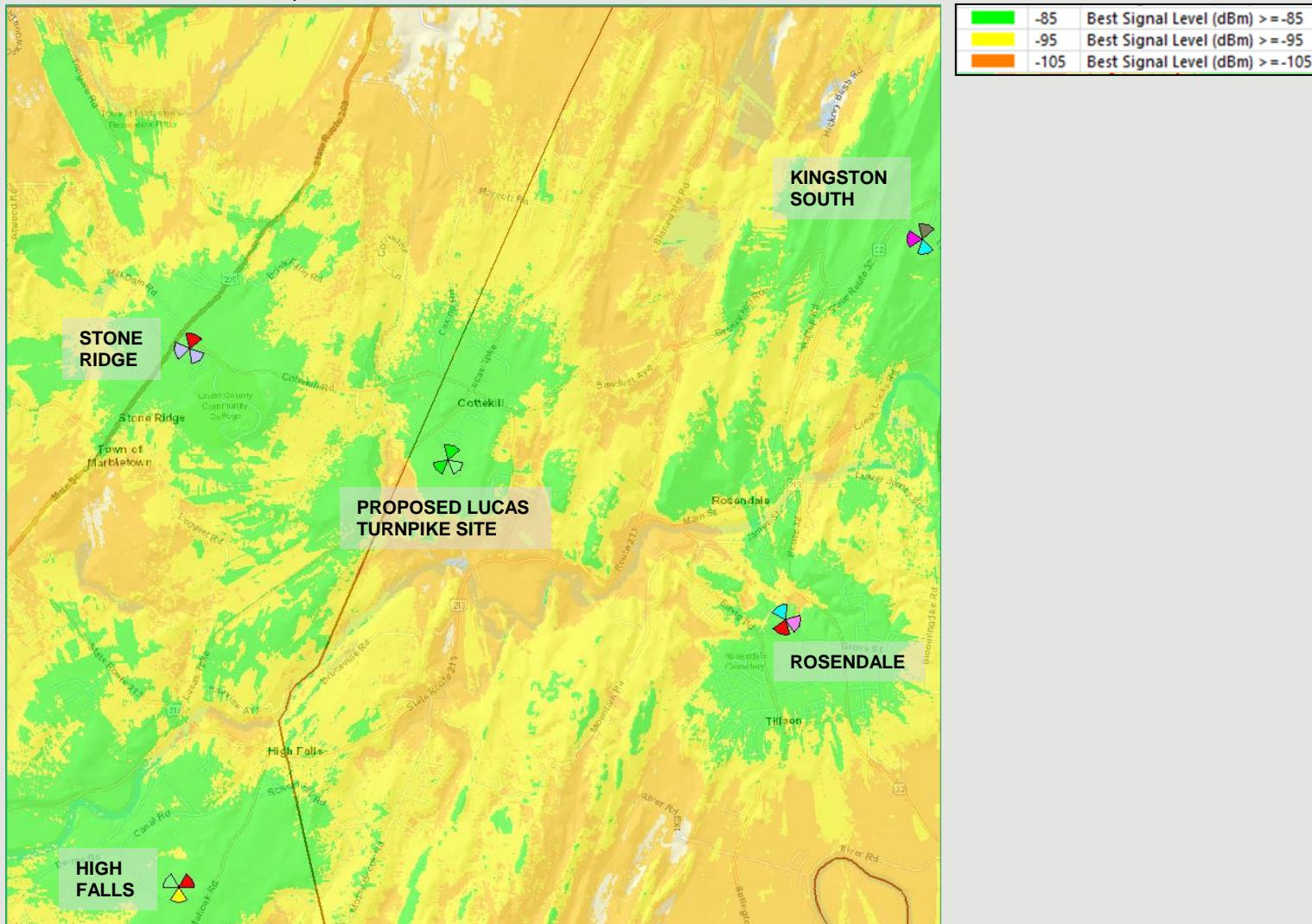
The map above adds low band of the **Lucas Turnpike** site to the existing signal strength. The significantly improved signal strength corresponds to improved coverage and capacity throughout the identified significant gap areas. This will help to resolve the coverage and capacity issues impacting portions of the Town of Rosendale.
